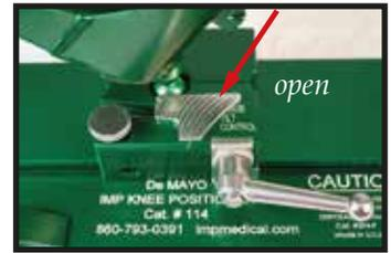
unlock the E-Brake by turning it counter clockwise,
