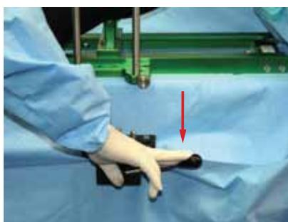
12. Rotate the lever to lock position requiring only 2 finger pressure. Works like a vice grip and “snaps” into place.
